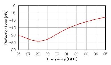
\*The absorption performance evaluation of radio wave absorber is based on our company's waveguide method and NRL arch method.
